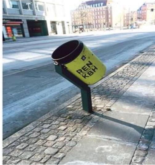
Trash cans in Copenhagen are angled so that cyclists can throw their trash while cycling.
