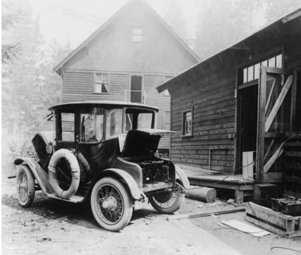
When the automobile economy looked so different Charging an electric car in 1905
